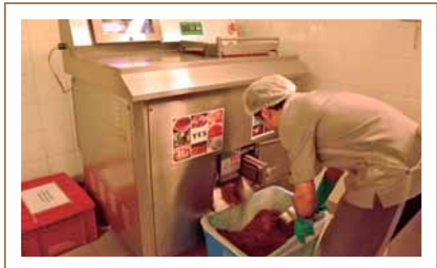
The compressed and dehydrated food waste is then placed inside the decomposing machine, which produces composites for landscape planting at Galaxy Macau™
